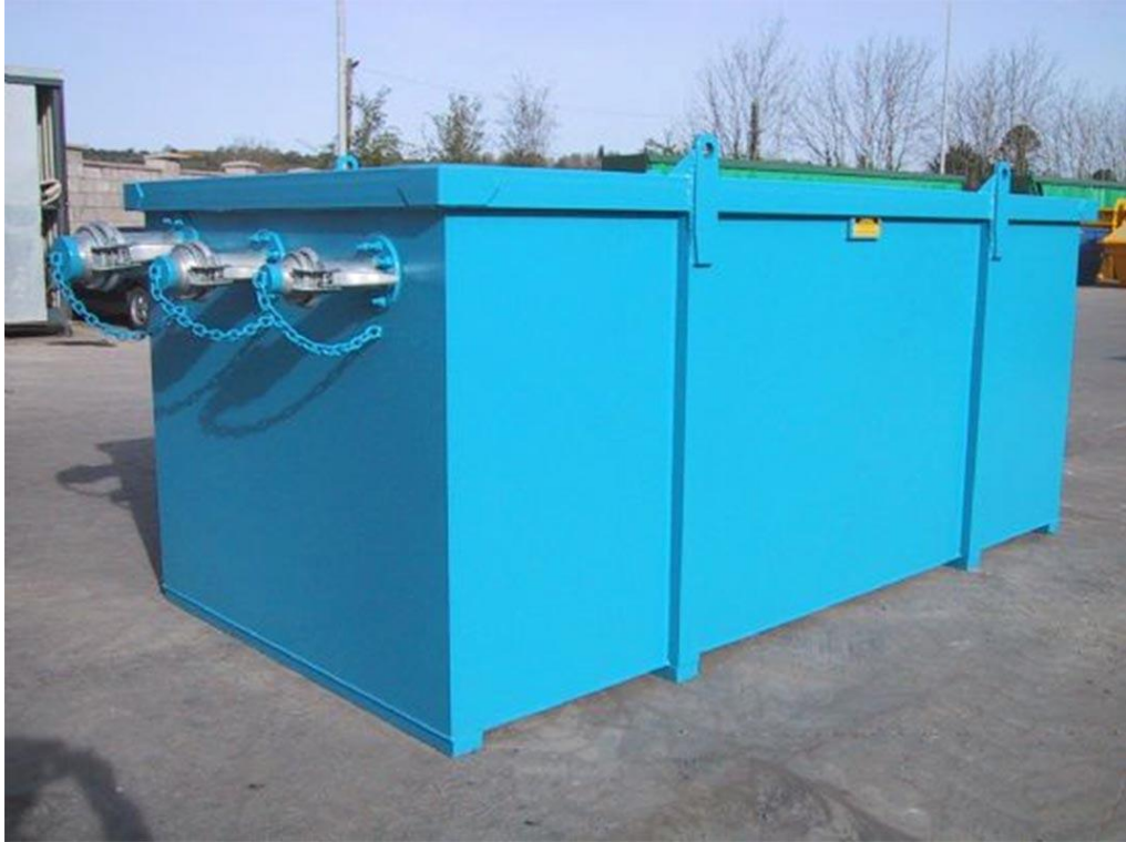
Figure 3.2f Example of Temporary Sediment Settlement Tank
